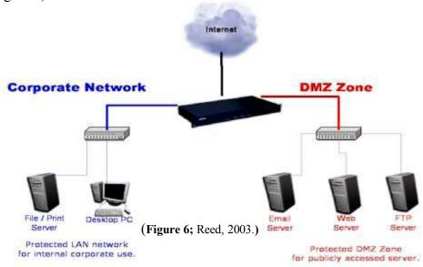
The "DMZ" enhances safety by keeping malicious outsiders on the Internet from accessing the private network. The safety and security of networks can significantly be enhanced through the proper combinatorial use of firewalls and demilitarized zones.
